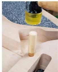
The bridge post mounting holes are drilled ready for the pivot screw bushings. Press in the brass bushings using The chuck in a drill press or If you dont have a drill press then you can hammer the bushings in taking care not to damage the brass inserts or their threads. Using a dowel will help with this and it will protect the surface of the body when driving them home flush with the surface.
