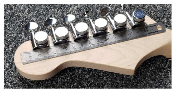
Mark out your mounting holes with a scribe or punch. Tuner mounting screws are very delicate, and will break off if forced into hard maple. Use a 5/64" drill bit to make pilot holes for the screws; if these holes are any smaller you risk shearing off the screw heads.
