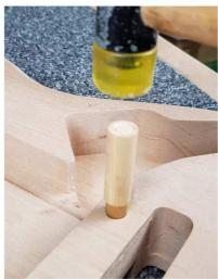
The bridge post mounting holes are drilled ready for the pivot screw bushings. Press in the brass bushings using The chuck in a drill press or If you dont have a drill press then you can hammer the bushings in taking care not to damage the brass inserts or their threads. Using a dowel will help with this and it will protect the surface of the body when driving them home flush with the surface.
